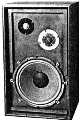
With the textured grille-cloth frame removed, the three drivers of the Sylvania AS125W are revealed. The tweeter dome is at upper left. The grille-protected mid-range is below it, with the 12-inch woofer at the bottom.
